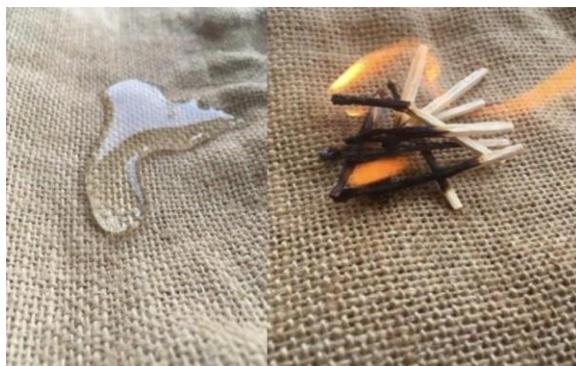
**Figure 4.** Jute Fabric is both Waterproof and Fire Retardant.
