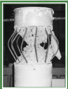
Figure 3. Column failure due to insufficient confinement
