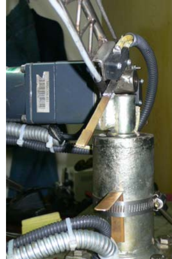
Figure 8. Switch that controls the downward movement
