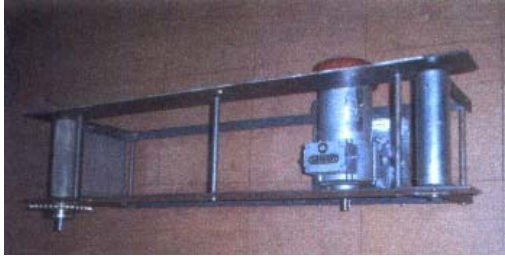
Figure 3. Conveyor Frame with the Motor
