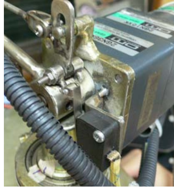
Figure 7. Switch that limits the upward movement
