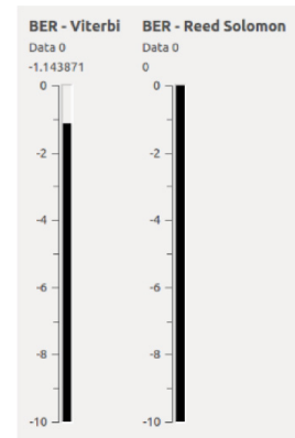
Fig. 12. BER of the Raw Baseband ISDB-T Signal (Convolutional Rate ≠ 3/4)
