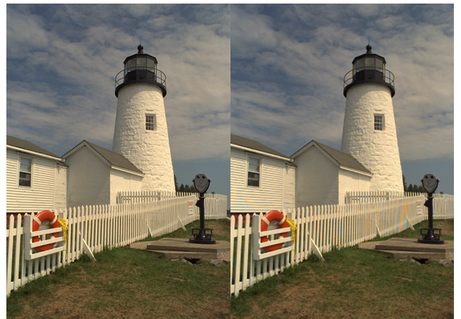
Fig. 3. Reconstruction of a mosaiced image using bicubic interpolation. Naïve interpolation can lead to color artifacts in the reconstructed image (right) that are not present in the original image (left).
